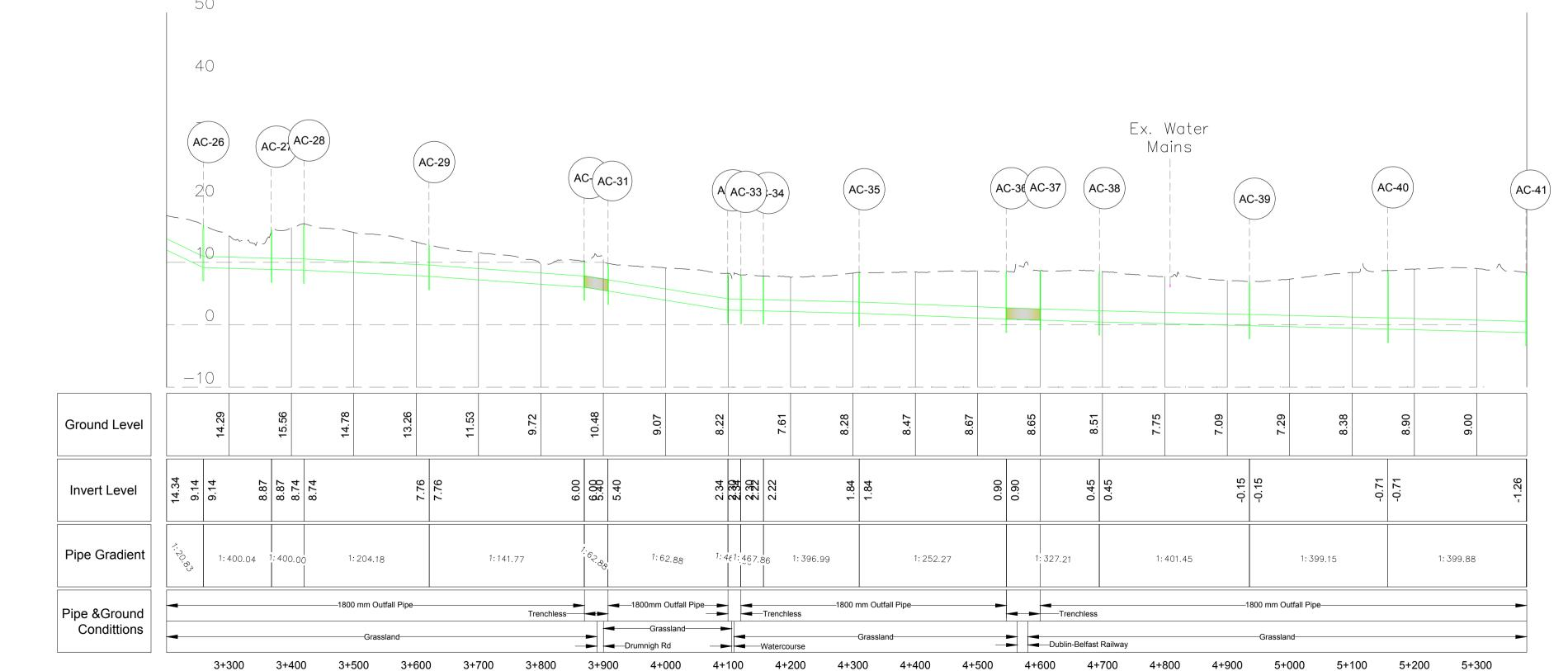
PROPOSED OUTFALL PIPELINE (LAND BASED SECTION)
